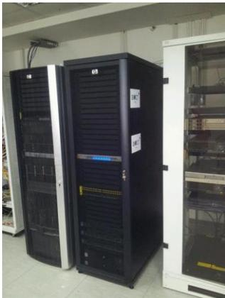
Pica8 and HP Procurve actually introduce a full network of OpenFlow switches to the testbed. HP Procurve has 24 1Gbps interfaces and 4 SFP+ optical transceivers. Pica8 is equipped with 48 1Gbps ports and 4 SFP+ optical transceivers. The same optical transceivers are part of NetFPGA-10G programmable boards.
